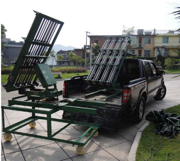
Fig. 2. Mobile rocket launchers used for precipitation enhancement.
